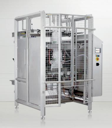
The ES400 is our ultra-sanitary, tough-as-nails fully stainless steel VFFS machine and can withstand the harshest washdown procedures. This servo-driven bagger is perfect for packaging fresh and frozen fruit, vegetables, and meat/poultry.
