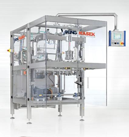
We offer a broad range of carton formers for lock or glue applications. The CFM machine is a rugged, versatile and high-performing carton erector, capable of running different carton shapes in single, double or triple head operation. The CFM machine provides state-of-the-art carton forming technology.
