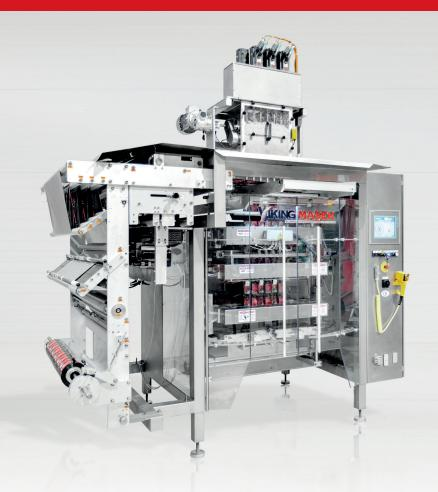
Viking Masek's SA300 is an intermittent motion sachet machine and is available with servo auger, volumetric or liquid fillers, to produce attractive 4-side seal sachets using just one roll of packaging film up to 600 mm wide.
