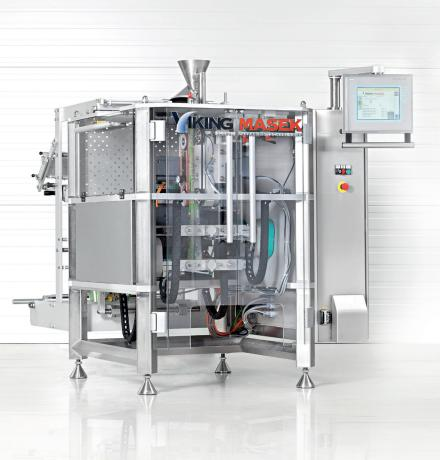
Patented, independently phased, twin sealing jaws separate the Velocity from all other high speed machines, and virtually eliminate lost cycle time. This is the fastest VFFS machine in the world – no competition.
