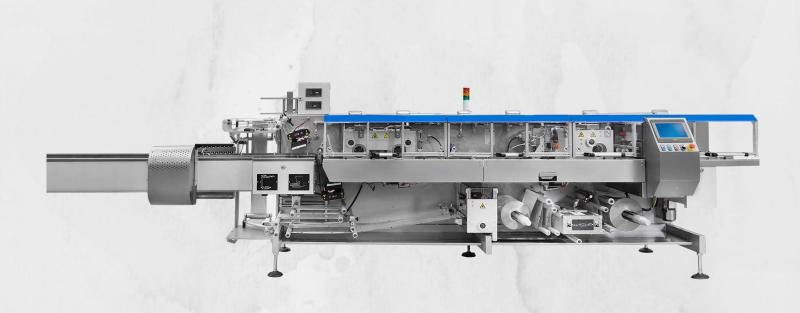
The FW-300 (top & bottom film reel holder) is the complete solution for a large variety of products with various production run speeds. Including semi-automatic or automatic feeding and multiple format changes.
