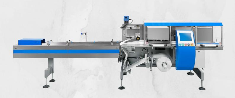
The FW-60 (bottom film reel holder) servodriven machine is the ideal solution for irregular, fragile, frozen, sticky or difficult to move products.
